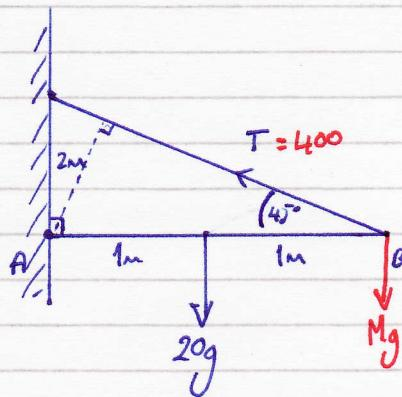
$$(a) \text{ At } C_a: 20g \times 1 - 2T \sin 45^\circ = 0$$
