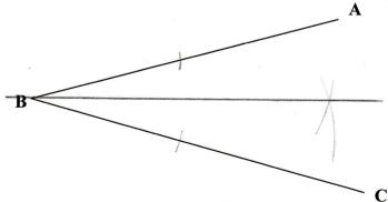
() Place compares point on B and open a reasonable distance. (2) Mark where company corres each line. (3) Without adjusting compares, place point on First mark. Prin an are. (4) Move compars point on second mark, drew an are which cross Firstarc. (5) The live through the intersection of the three lives and area is the angle birector
